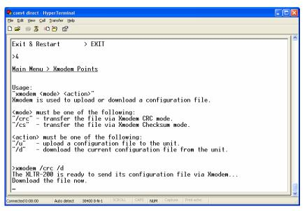
Figure 22: "Xmodem" Command Overview and Implementation
